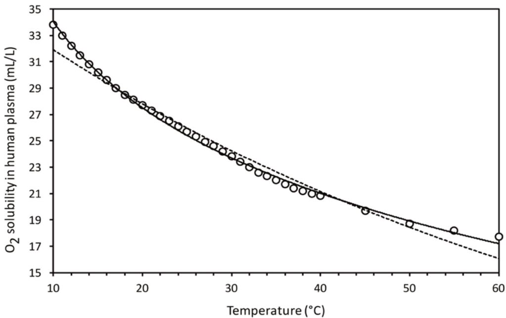
**Figure 1.** Solubility of oxygen in human plasma  $X_{O_2}$  [mL(gas)/L(fluid)] at standard atmospheric pressure. Circles: experimental data by Christoforides et al. [1969]; continuous line: logarithmic interpolation; dashed line: exponential interpolation.
