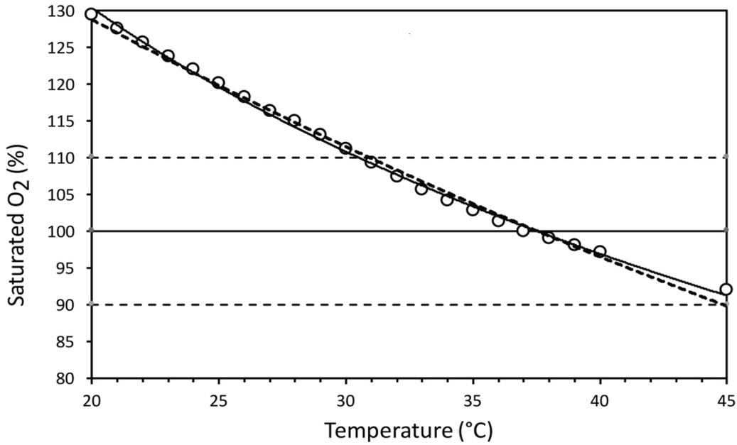
**Figure 2.** Saturation level of the oxygen dissolved in human plasma at various temperatures, referring to the value at 37° C, assumed to be 100%. Circles: saturation of experimental data; continuous line: logarithmic interpolation; dashed line: exponential interpolation. Horizontal lines pinpoint the 90, 100 and 110% levels.
