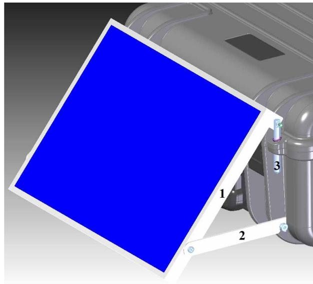
**Figure 3.** Fixing system of the photovoltaic panel to the suitcase, during the acquisition configuration.
