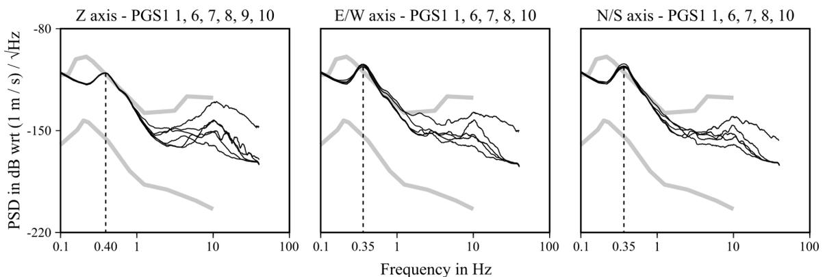
Figure 10. Power Spectral Densities from the recordings made in the Sulcis, in 2017. The horizontal components from station PGS1 9 are not included, because the corresponding time series are affected by strong noise, in the form of a train of periodic pulses, which prevents the correct evaluation of the spectra. The cause of this noise was a faulty electrical connection, inside PGS1 9.
