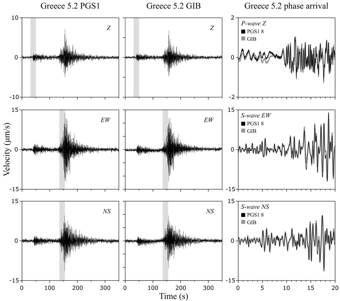
**Figure 13.** Earthquake of magnitude 5.2, occurred in Greece on Oct 1st 2020, UTC time 11:05:37, as recorded by PGS1 n°8 and by the seismic station Gibilmanna (code GIB).
