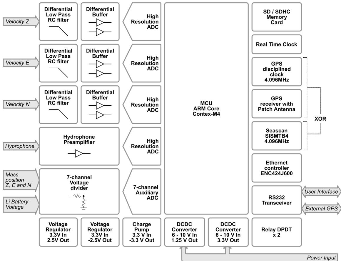
Figure 5. Simplified system diagram for the SeismoLog recorder.
