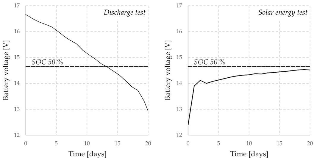
**Figure 8.** The graph on the left shows the voltage across the Lithium battery pack during a 20-days uninterrupted recording, with one battery pack and without photovoltaic panel. The graph on the right shows what happened when the photovoltaic panel was connected. The horizontal line labeled SOC 50% shows the point where the battery charge (State Of Charge, or SOC) is 50%.
