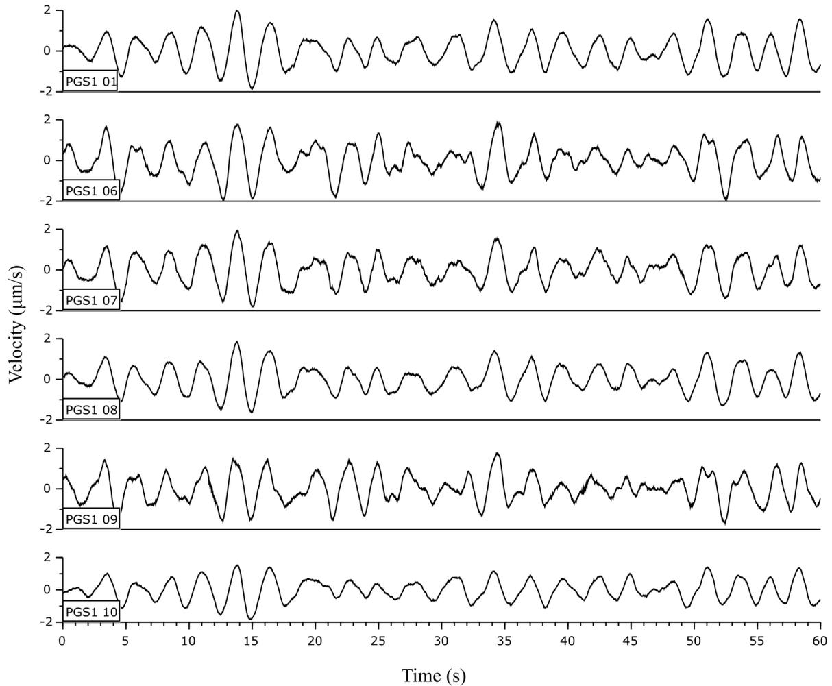
**Figure 11.** Ambient noise recorded in Sulcis in 2017. Only the E/W axis is shown. The time series produced by PGS1 9 are affected by strong noise, in the form of a train of periodic pulses, due to a faulty electrical connection. The data segment above was chosen so that the pulses are not visible.
