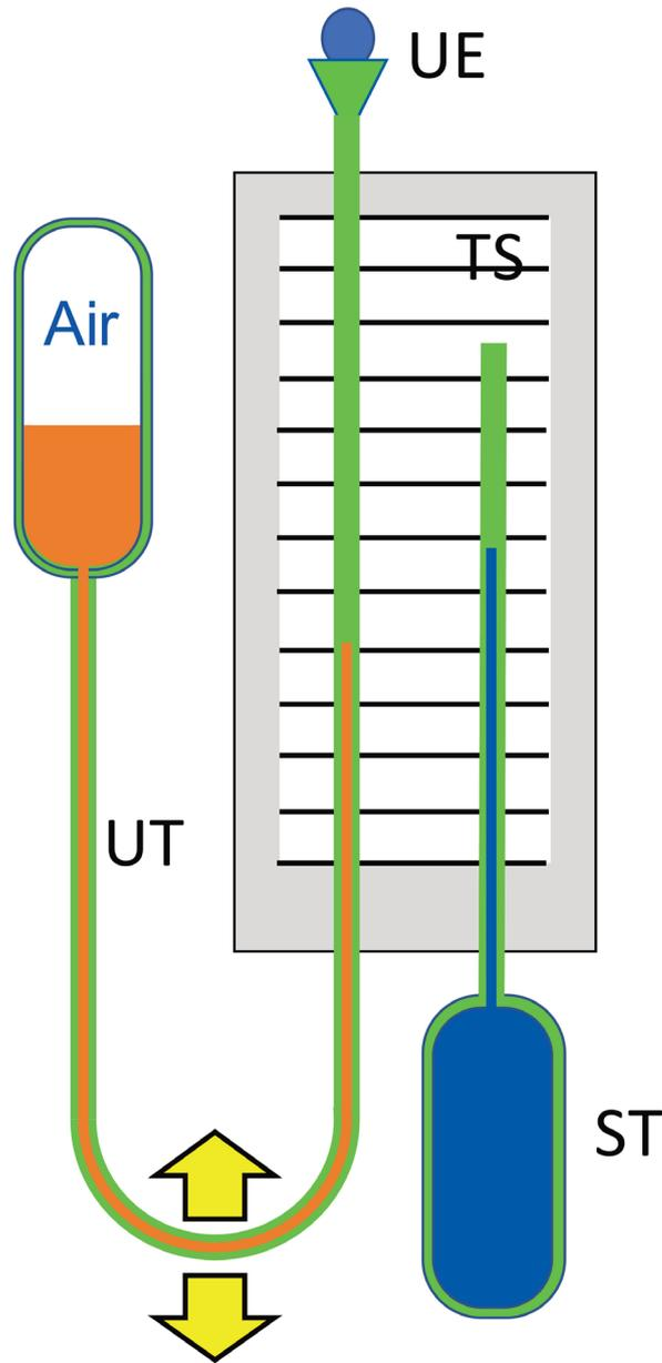
**Figure 5.** Scheme of the assembly constituted by the U-shaped device (UT) and the spirit thermometer (ST).
