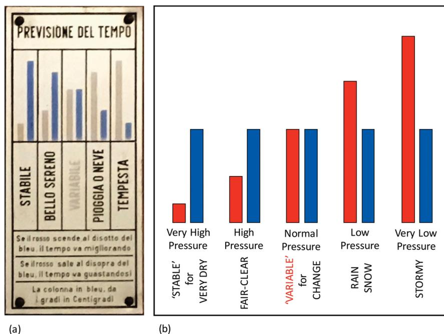
**Figure 3.** (a) The original instruction table (IT) where at each class the temperature (blue bar) is represented at different values from the highest to the lowest. This might be misleadingly interpreted from summer to winter. Red bars (now grey) represent the output of the UT tube. The red colour used in the bars and the heading «*variable*» has faded. (b) The same scheme, but redrawn making reference to temperature, always at the same level, to avoid misleading interpretation.
