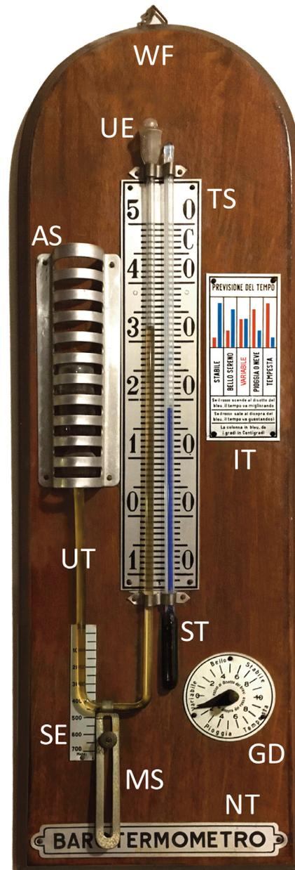
**Figure 1.** The *Barothermometer* (digitally restored) indicating 18.5° C and stormy weather. Letters to recognize the parts of which the instrument is composed (see text).
