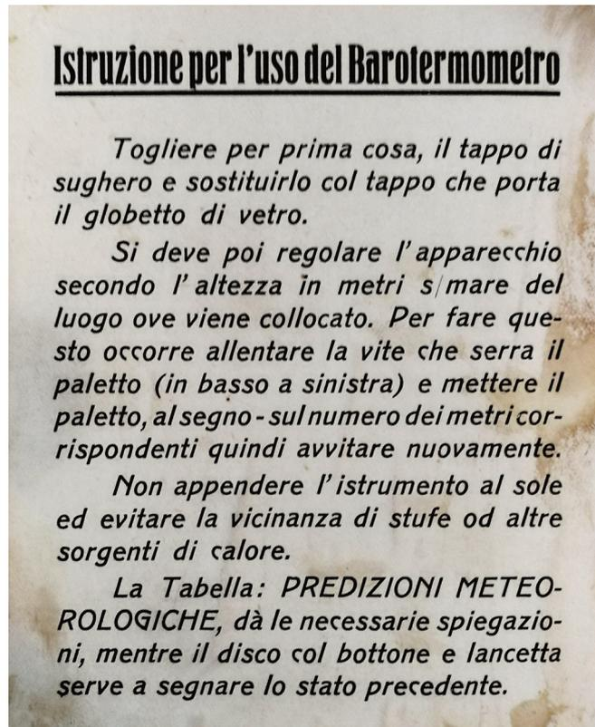
Figure 4. The paper sheet with instructions glued on the back of the frame.
