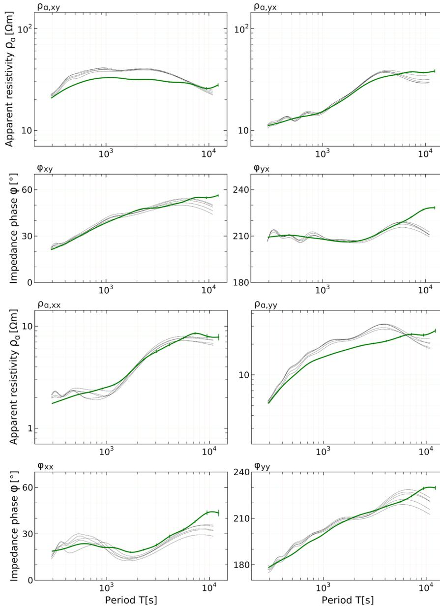
**Figure 5.** A comparison of the results of the transfer function estimation for data that fulfill (green color) and do not fulfill the plane wave assumptions (black).
