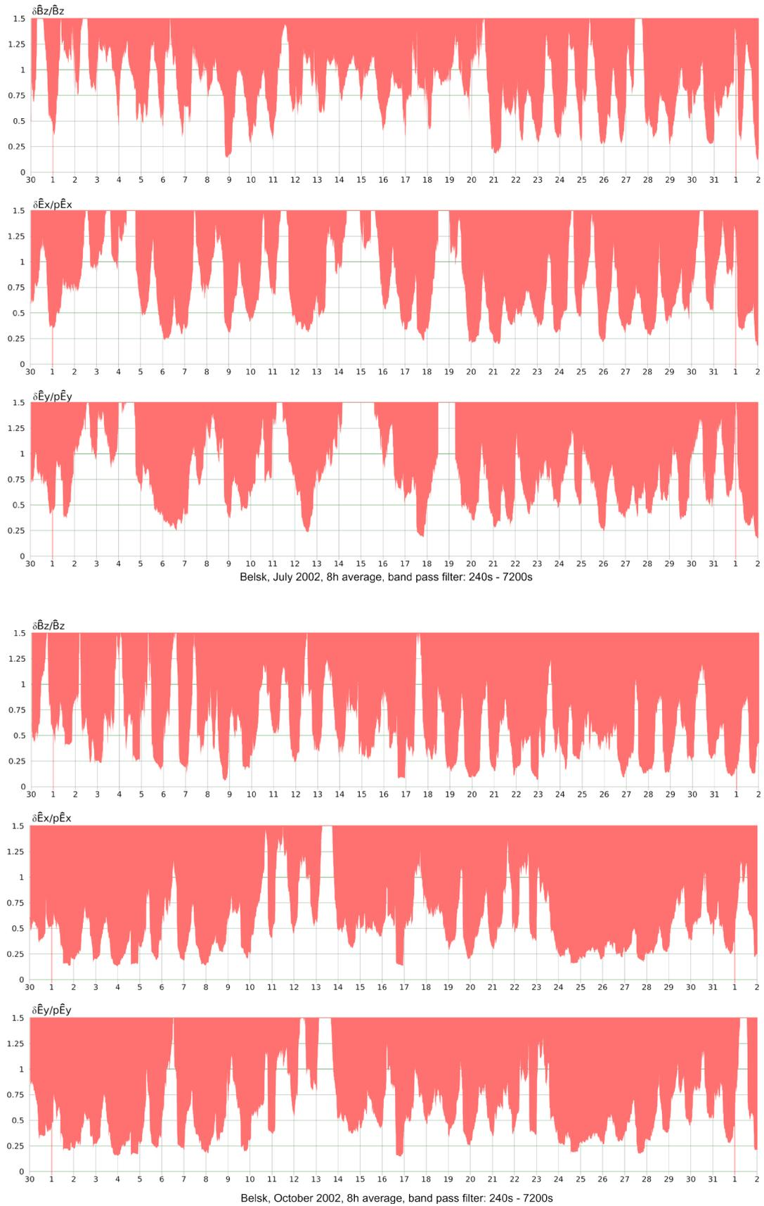
**Figure 3.** Plots of the ratio  $\delta\widehat{B}_z/\widehat{B}_z$ ,  $\delta\widehat{E}_x/p\widehat{E}_x$  and  $\delta\widehat{E}_y/p\widehat{E}_y$  (moving averages over periods from 240s to 7200s in the frequency domain) as a function of time. Length of moving intervals is 8 hours each, with 1 min sampling rate. To enhance the readability of the diagram, values exceeding 1.5 (150% error) are truncated, and the areas in excess of the function value are shaded red.
