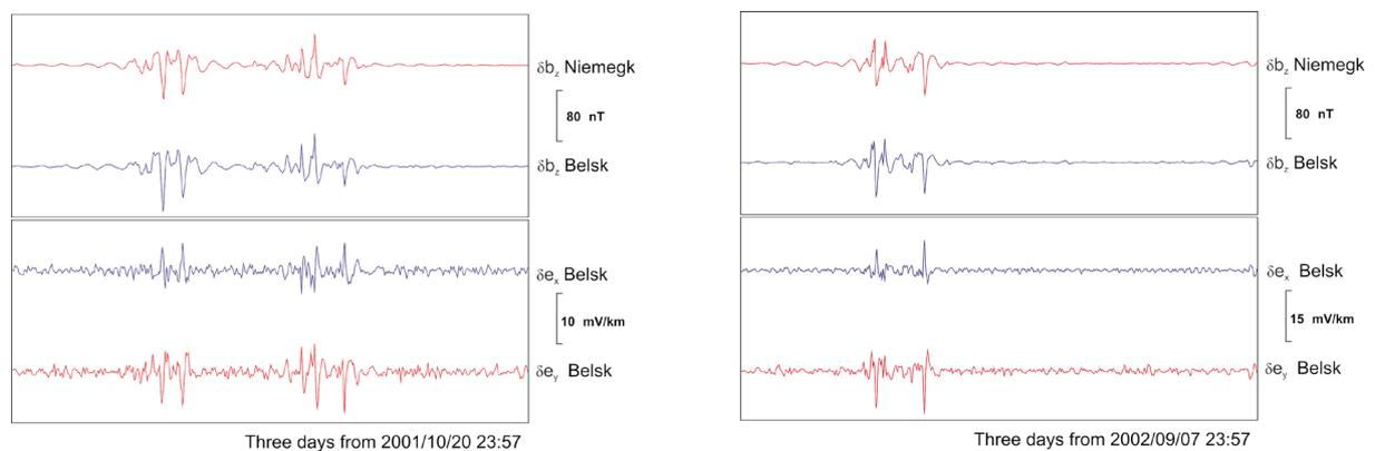
**Figure 4.** Samples of data with the external field deviating from plane waves in the form of 3-day time series; the top two curves are  $\delta b_z(t)$  for the observatories in Niemegek and Belsk; the two lower curves are errors in the predictions of the telluric components  $\delta e_x$  and  $\delta e_y$ .
