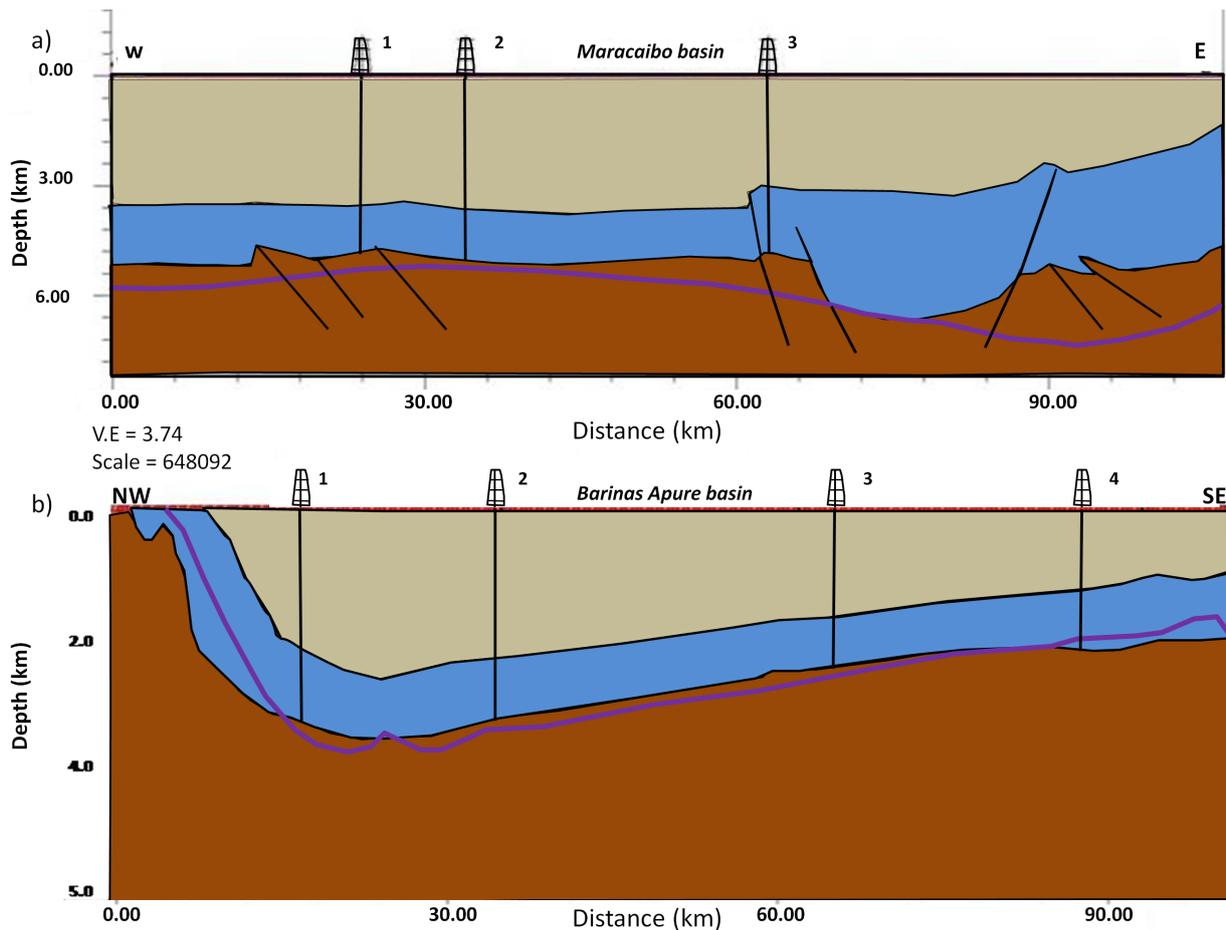
**Figure 6.** Comparison between the basement depth from gravimetric inversion (purple line) and the basement given by two seismic reflection lines (see figure 1 for the location of profiles 6a and 6b). The wells reach the metamorphic igneous basement located in Maracaibo Lake basin and Apure Barinas basin. Seismic line above [Escalona and Mann, 2003] below [Parnaud et al., 1995]
