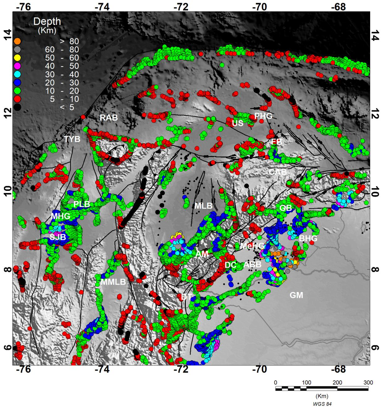
**Figure 10.** Euler deconvolution in western Venezuela and northern Colombia, the range of depths goes from 5 km to greater than 80 km, with red (5-10 km depth) and green (10-20 km depth) being the dominant depth ranges.
