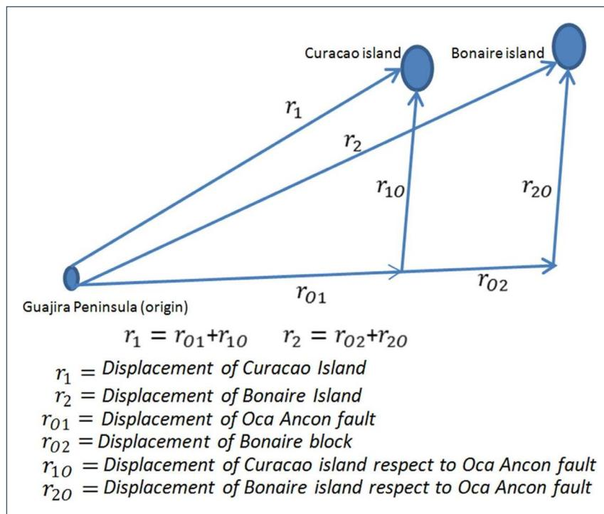
**Figure 8.** Vector diagram associated with the movement of the Oca Ancon fault, Aruba Bonaire Island and the Bonaire block. The  $r_1$  represents the distance between the Guajira Peninsula (origin) and Morrocoy fault or Curacao island,  $r_2$  distance between origin and Bonaire island,  $r_{01}$  is the displacement of Oca Ancon fault,  $r_{02}$  displacement of Bonaire block,  $r_{10}$  and  $r_{20}$  is the displacement of Curacao, Bonaire respect to Oca Ancon fault.
