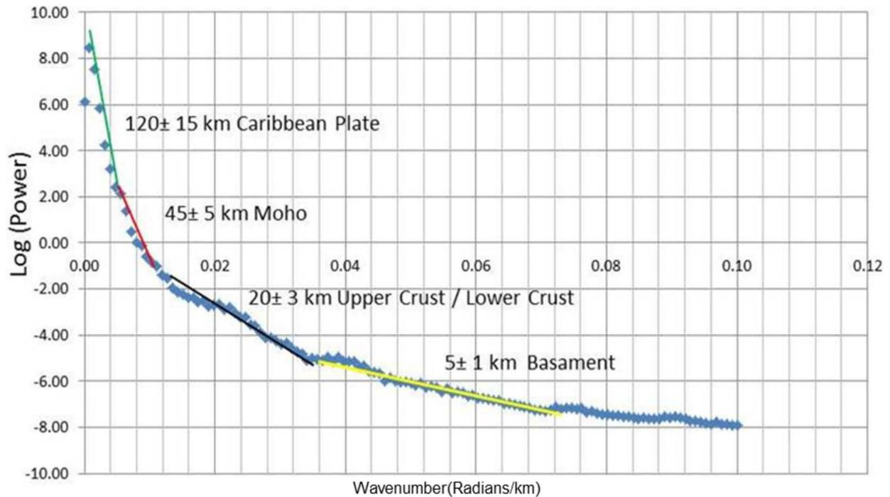
**Figure 3.** Radially averaged power spectrum of the CBA showing the source depths estimated from the slopes of the curve. The largest wavelength components are most likely associated with Caribbean plate and the Moho discontinuity, the mid wavelength component with the lower crust/upper crust boundary and, the shortest one, with the basement.
