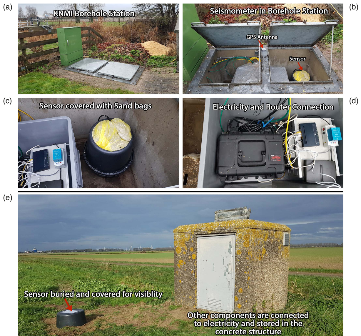
Figure 7. (a-d) Example of deployment of station NE411 in a KNMI Borehole location where the seismometer is placed in the existing safe facility and connected to electricity supply. All the components of the stations are placed in the instrument vault, except the GPS antenna, which is placed at the top for proper signal reception. (e) Example of deployment of station NE418 at a KNMI automatic weather station. The sensor is buried in a tube installation in the ground and covered with black plastic for visibility. Other components are connected to electricity supply and stored in the weather station.
