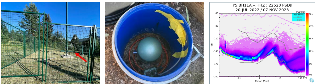
Figure A11. BH11A, Klekovača, is installed in an open free-field in a mountainous area. The sensor is installed in a self-constructed seismic vault within a fenced area built for a meteorological station and rests on a self-constructed concrete foundation. Due to the swaying of the mast in the wind, we observe periodic degradation of the long-period signal.
