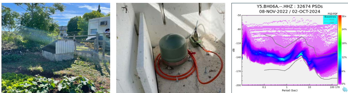
Figure A6. BH06A, Kalinovik, is installed in an urban free-field. The sensor is placed on a concrete pedestal inside a seismic vault on the periphery of a small village. The sedimentary setting at this site causes higher noise levels compared with the sites on crystalline rock.
