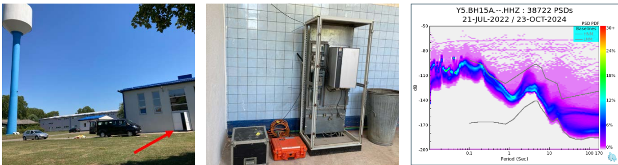
Figure A15. BH15A, Šamac, is installed in a two-storey building (6 m × 12 m) used as a machine room for a local water reservoir in a small village. The sensor is located on the ground floor in the northern part of the building and placed directly on the concrete floor. Due to the swaying of the nearby mast in the wind, we observe periodic degradation of the long-period signal.
