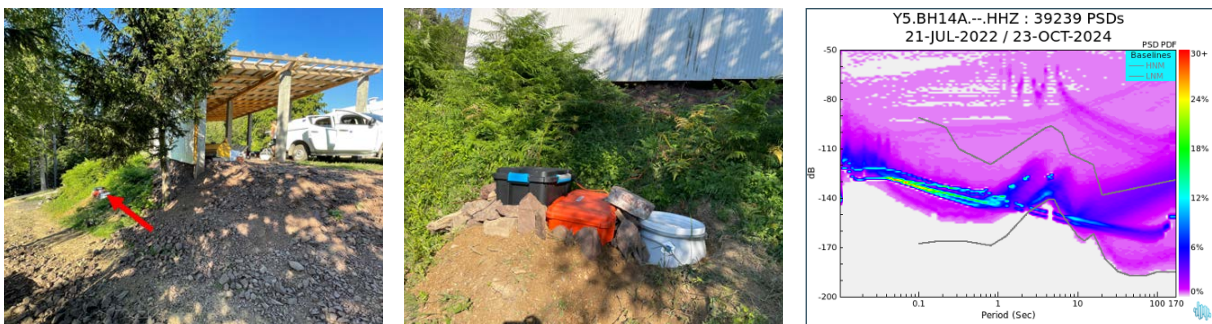
Figure A14. BH14A, Ocaus, is installed in an urban free-field. The sensor is inside a self-constructed seismic vault at a distance of 10 m from a one-storey building less than 8 m high. It is placed on a self-constructed concrete foundation on a relatively steep slope with soil ground. The sedimentary setting at this site causes higher noise levels compared with the sites on crystalline rock.
