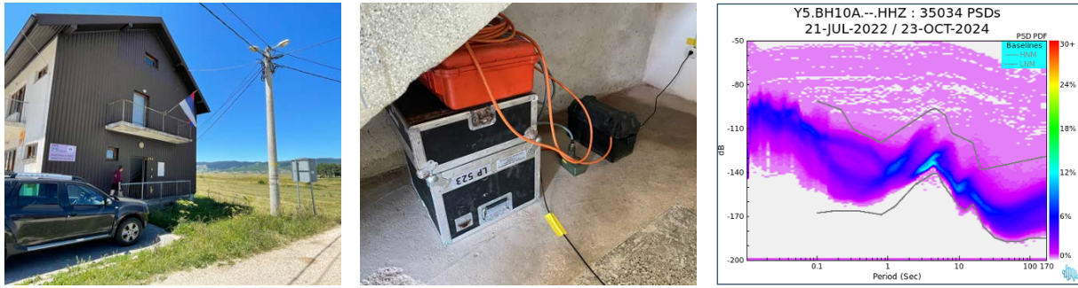
Figure A10. BH10A, Kupres, is installed in a used municipal office. The sensor is in the basement, in the north-central part of a two-storey building. It is placed directly on the concrete floor.
