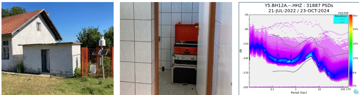
Figure A12. BH12A, Magaljdol, is installed in a small building (former toilet) with a 4 m × 2 m footprint, 2 m away from a one-storey abandoned school. The sensor is on the ground floor, in the southeast corner of the room, placed on floor tiles. This station is solar-powered.
