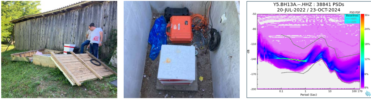
Figure A13. BH13A, Krupa na Uni, is installed in an urban free-field, housed in a seismic vault. The sensor is placed on a concrete pedestal, 5 m from a one-storey building. The sedimentary setting at this site causes higher noise levels compared with the sites on crystalline rock.
