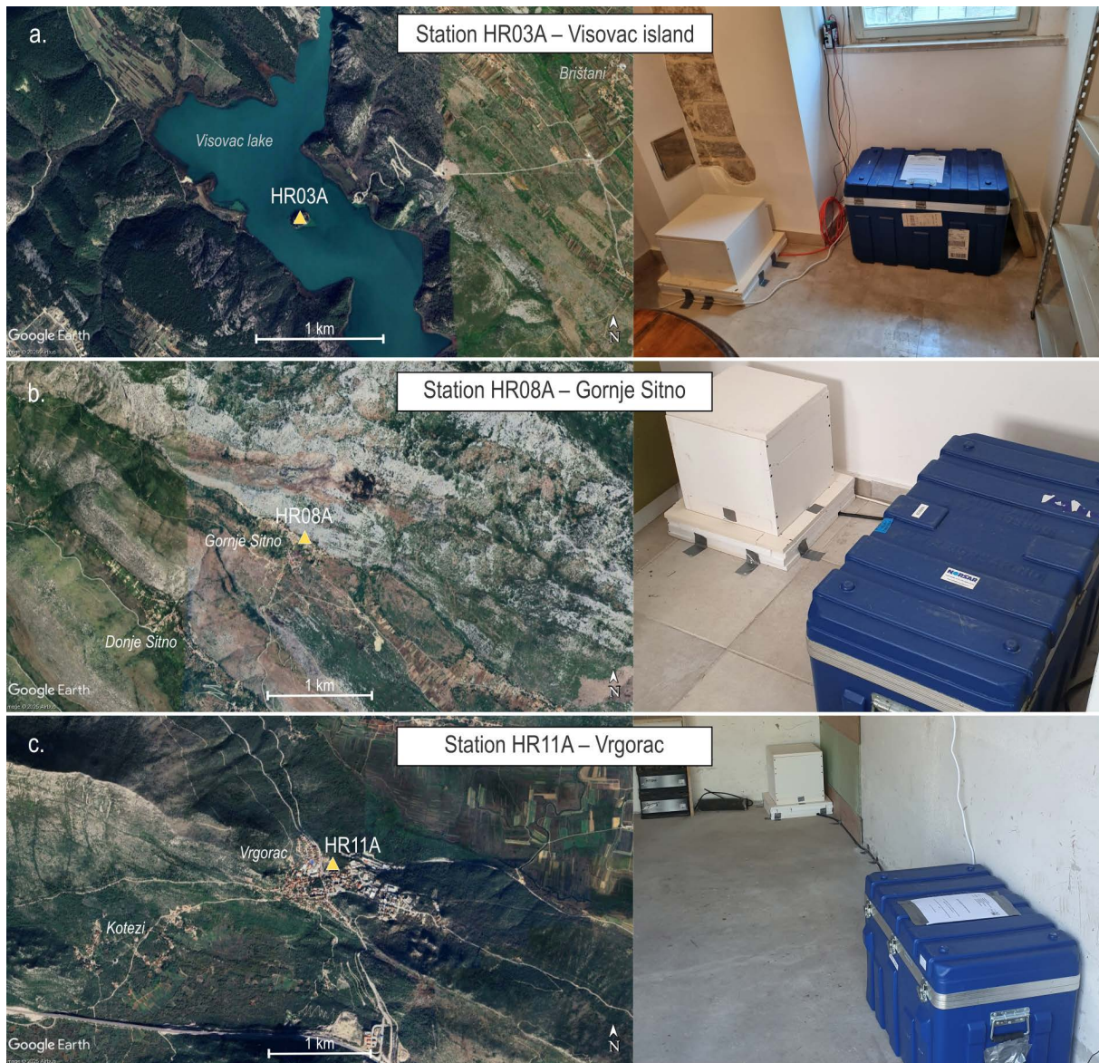
Figure 2. Examples of site location and installation configurations for three seismic stations (rows). Pictures to the left show the station's position on Google Earth (yellow triangles). Pictures to the right display photographs of each installation site in the building that hosts the instruments. The stations are (a) HR03A in a Franciscan monastery on Visovac island in Visovac lake (National Park Krka); (b) HR08A in a small school in the mountain village Gornje Sitno, 14 km from the Split's city centre; (c) HR11A in the small town of Vrgorac.
