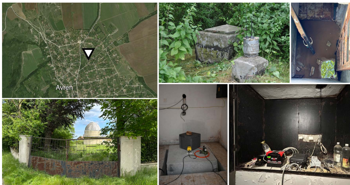
Figure 7. Installation of the broadband seismometer and data acquisition system GAIA at station AVR in the Astronomical Observatory in Avren.
