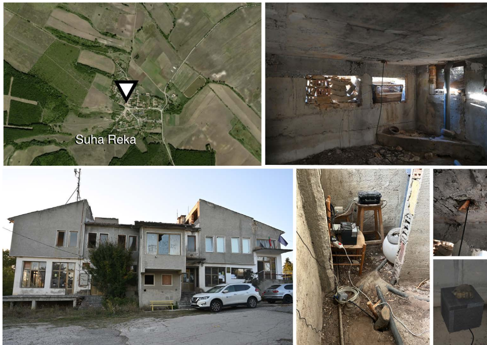
Figure 6. An example of station installation in municipality building: station BG03A at Suha Reka.
