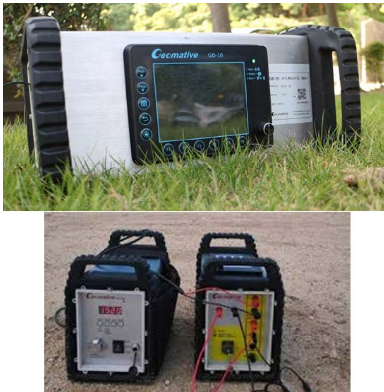
Figure 4. Geoelectrical System equipment, model GD10, manufactured by Geomative.
