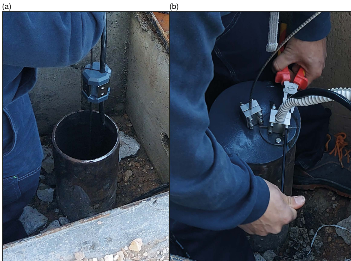
Figure 7. (a) Details of the cable ties during the descent of the sensor into the steel casing. (b) Steel cap that supports the cable ties for the data cable and the lifting cable.
