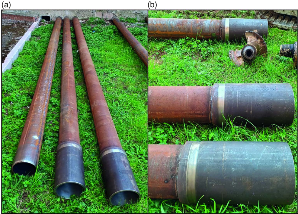
Figure 5. (a) Segments of the steel pipe. (b) Details of welded joints used to join different pipe segments.
