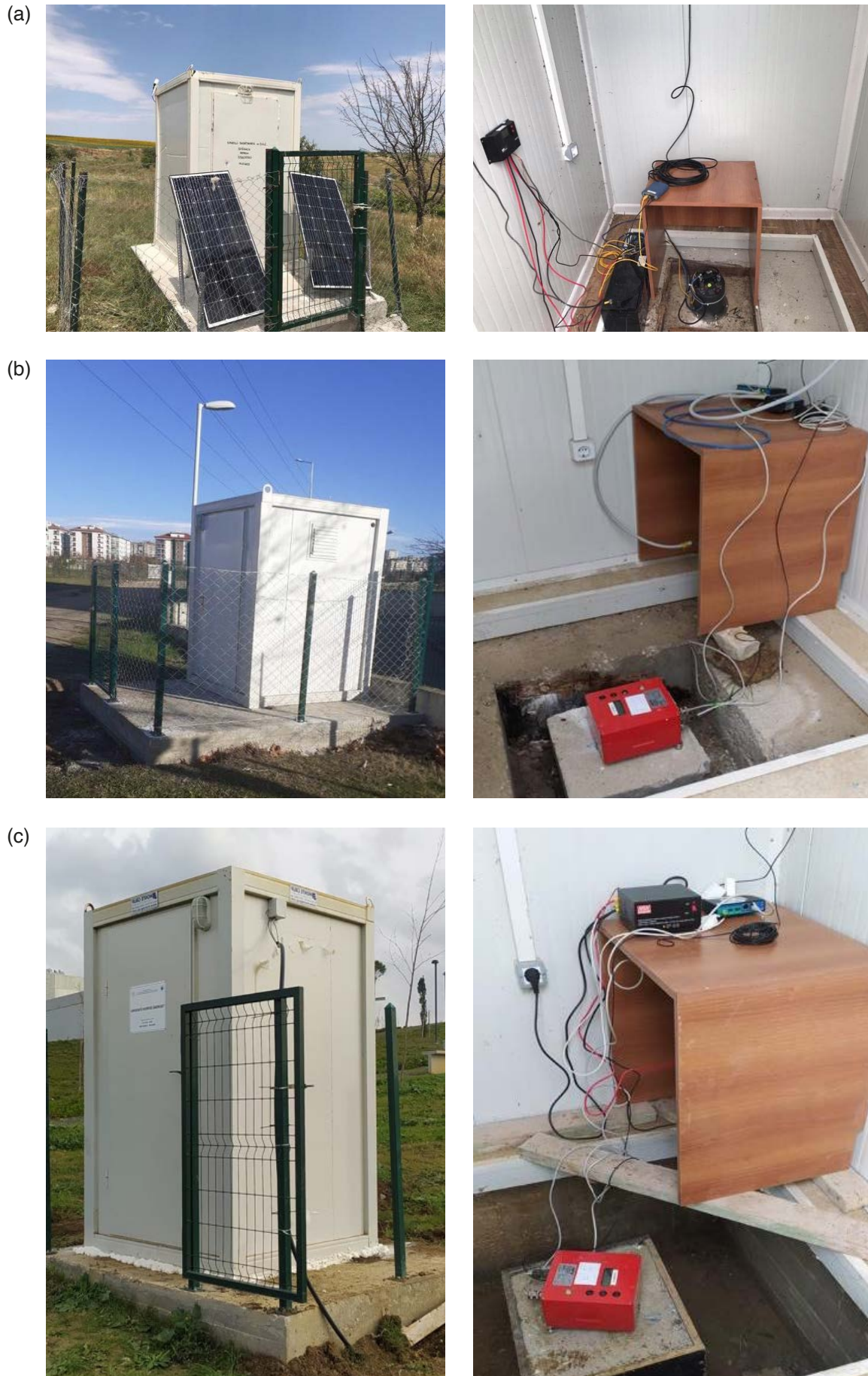
Figure2. Installation and Overview of the AdriaArray Stations; (a) DOGC, (b) CRLU and (c) TEKI.
