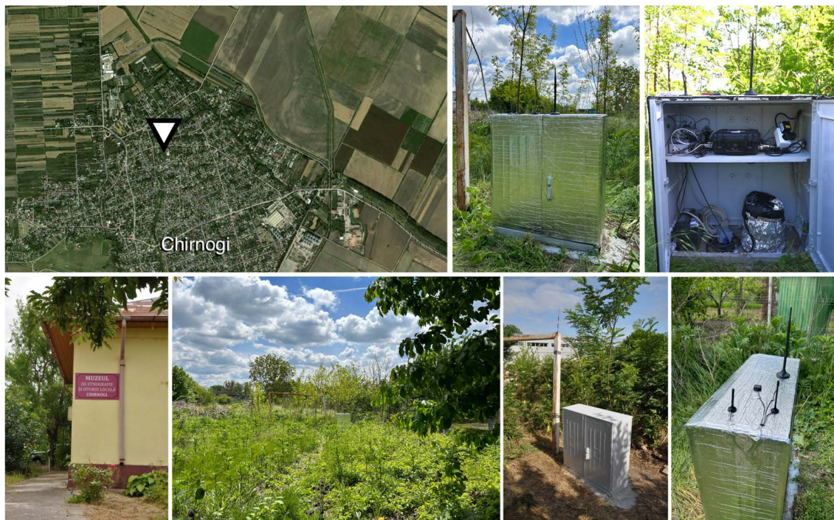
Figure 4. Location of the RO16A temporary station in the yard of the local museum in Chirnogi, with an overview of the surrounding area. The plastic enclosure (non-isolated/isolated), isolated broadband seismometer, data acquisition system GAIA, and communication system are shown.
