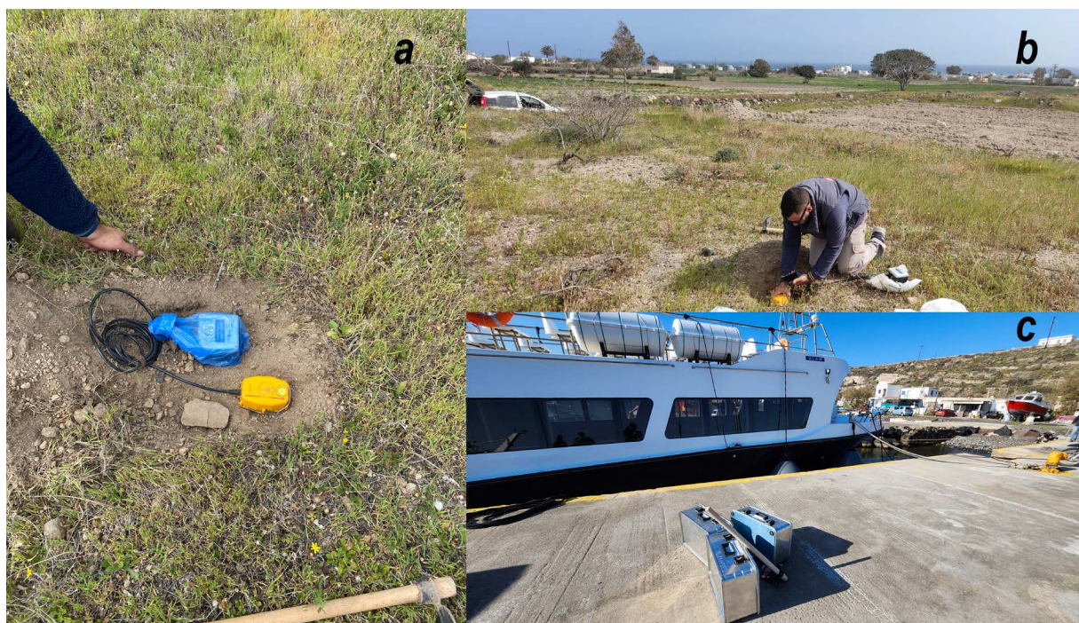
Figure 3. Example field site installations: (a) Typical sensor and DATA-CUBE placement, (b) Station STA40 site deployed in the Vlychada-Perissa area (see Fig. 2b), (c) Boat transportation of instrument boxes to the Thirasia and Nea Kameni islands.
