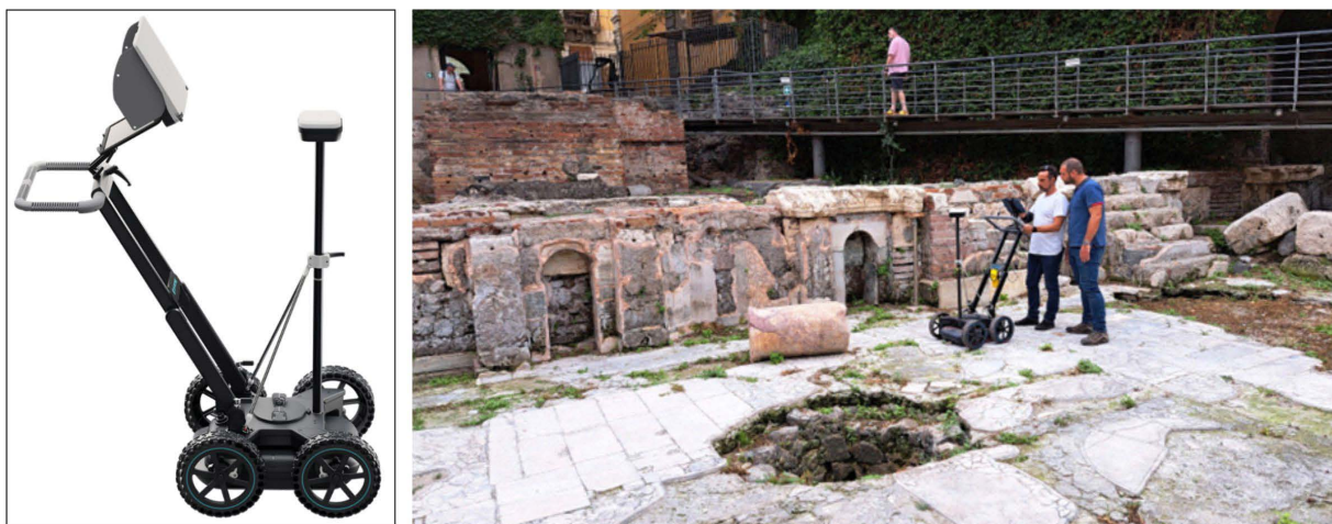
Figure 5. Ground-penetrating radar equipment used and survey phase.
