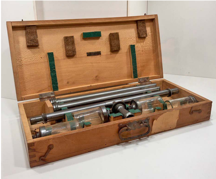
Figure 2. Water level, signed R. Radaelli, Milan, Italy, first half of the 20 th century. The water level is based on the principle of equilibrium in communicating vessels. When placed horizontally and filled with water, the liquid rose to the same height in both glass containers. Equipped with adjustable and measurable sights, the instrument was used to calculate the difference in elevation between two points. It proved particularly important for measuring the new morphological configuration after eruptions of Mount Etna. Museum of Mineralogy, Petrography, and Volcanology. University of Catania. General catalogue number: Instrument_52.
