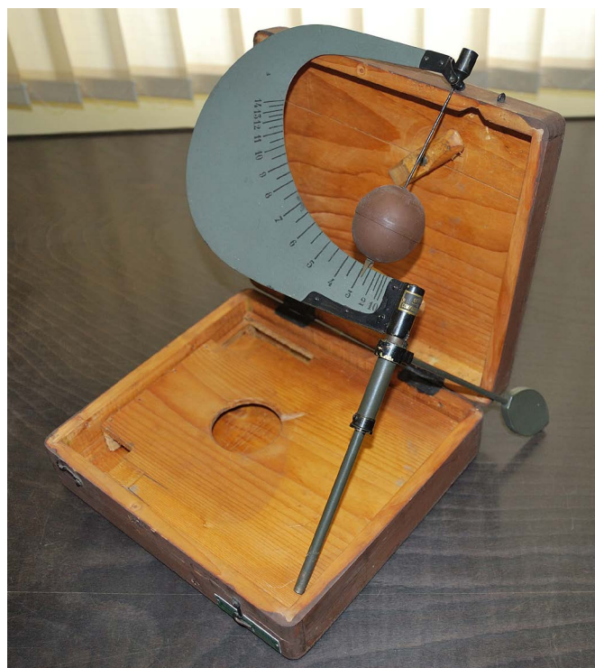
Figure 6. Daloz-type anemometer, signed Officine Compagnia Speciale X, Italy, first half of the 20 th century. Its operating principle is based on the deflection of a lightweight sphere, attached to a pendulum mounted on a horseshoe-shaped aluminum alloy bracket. A horizontal counterweight balances the system. The rod supporting the sphere features an indicator needle, which points to the wind speed, expressed in meters per second (m/s), on a graduated scale engraved directly onto the bracket, ranging from 0 to 14 m/s. The sphere is affixed to a pendulum, which is itself mounted on a vane system that allowed the instrument to be oriented in the direction of the wind. As wind pressure acts upon the sphere, the pendulum tilts at an angle proportional to the equilibrium between the sphere’s weight and the aerodynamic force exerted by the wind. This angle directly indicates the wind speed. A label reading “Officine Compagnia Speciale X” is affixed to the instrument, likely referring to a unit of the Italian Army’s Engineering Corps specialized in chemical defense and active between 1916 and 1919. Museum of Mineralogy, Petrography, and Volcanology. University of Catania. General catalogue number: Instrument_42. Another exemplar of this kind is preserved at the Alpines Museum München.
