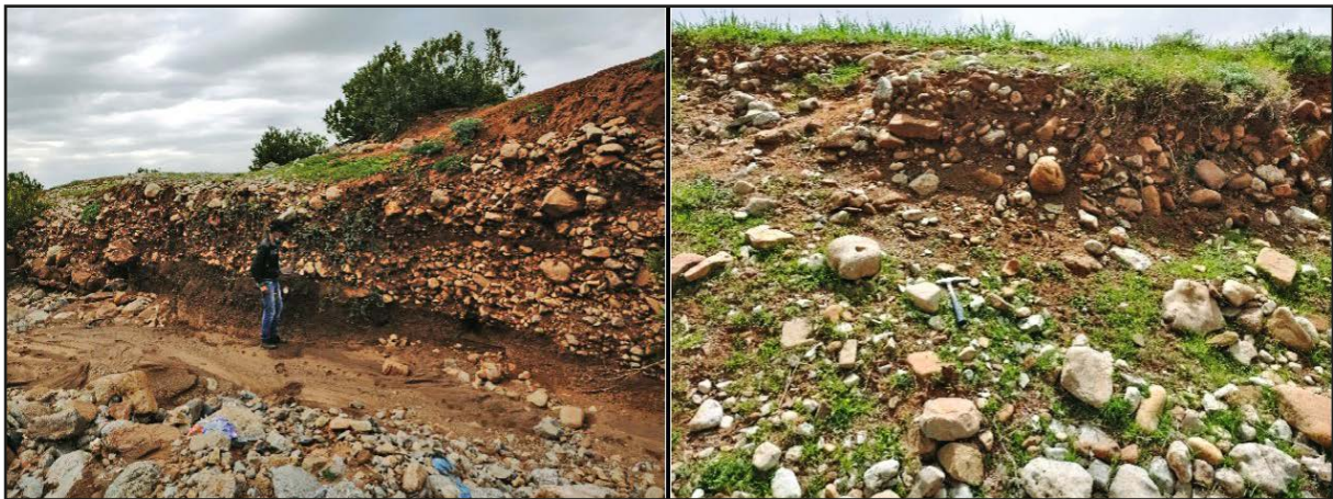
Figure 4. Photos illustrating the coarse silty-clayey conglomeratic facies that characterize the Quaternary terrace in the northeastern part of the study area.
