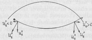
Fig. 8 - The changing of the sign of SV due to the curvature of the ray.
